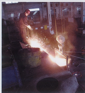
▲ 电炉熔炼 Electric furnace smelting
